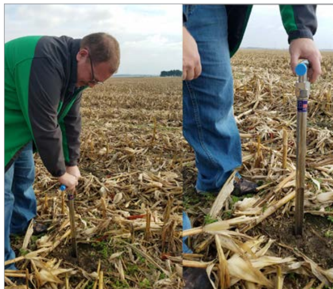
Figure 1. Collecting a soil sample with a soil probe. Insert the probe vertically into the soil and remove the soil core.
